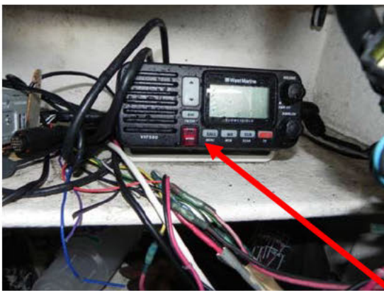
VHF Marine radio with weather channel, located in the steering console
