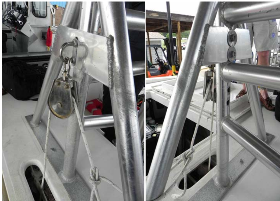
WHY KNOT's A-Frame. Investigators found the pulley's u-bolt nuts only hand tight and only a few turns from falling off.
