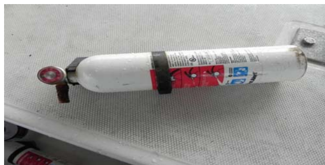
WHY KNOT's onboard portable fire extinguisher. Note the operational handle is broken off and missing.
