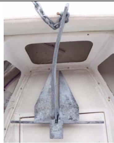
External force applied to WHY KNOT bent the anchor's shank and right fluk
